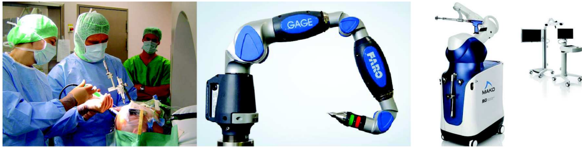
Figure 3.1: Left : Surgeons use a stereotactic frame to locate surgical targets during neurosurgery 1 ; Middle : FARO Gage 3D coordinate measurement arm, a hand-operated metrology tool that can find applications in precise registration of rigid targets 2 ; Right : Stryker MAKO co-manipulated orthopaedic surgery robot - knowledge of the kinematic linkage of the robot can allow for tracking of the tool-tip position in space 3 .
