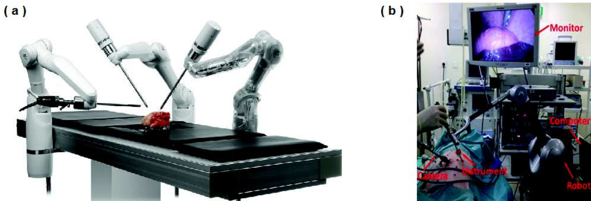
Figure 1.7: Examples of modular, large workspace RMAS solutions currently undergoing development: (a) the modular teleoperated robot arm system developed at DLR; (b) the Achille co-manipulator robot arm developed at ISIR.
