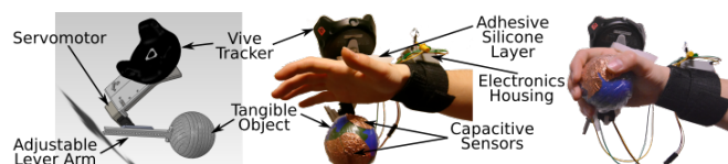
Fig. 1. The WeATaViX interface - From Left to Right: CAD assembly, disengaged device (free hand), engaged device (user grasps a virtual object)
